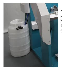
Water for the steam generator is contained in a 50 litres tank, supplied with the machine. Is also possible to connect directly to the water supply system.
