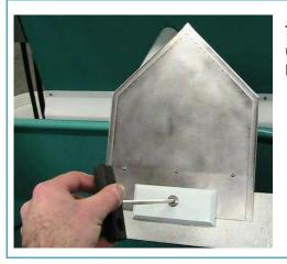
The format change is simple and fast, it only requires the unloosing of the screws and pulling out the plate from the holder.
