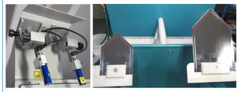
There are four red line optic lasers 2 for the small plate, and 2 for the big plate.
