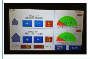
LCD touch screen panel for control the machine, the ironing programs, shows the functioning parameters, and allows to control all the functioning parameters of the machine.
